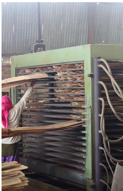
Veneer charged into the dryer on our own line.
